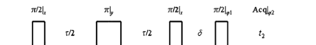
Fig. 1. RF pulse sequence for generating and detecting double quantum coherence used in this work. In the experiments the phases were \phi_1 = x, y, -x, -y and the acquisition phase \phi_2 = x, -y, -x, y . The phase cycle can be shown to only select double quantum coherence while suppressing zero and single quantum coherences [23,29].
